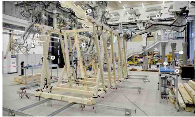
Figure 2: Robotic assembly system (Helmreich et al., 2022), with permission by Gramazio Kohler, ETH Zürich ©.
