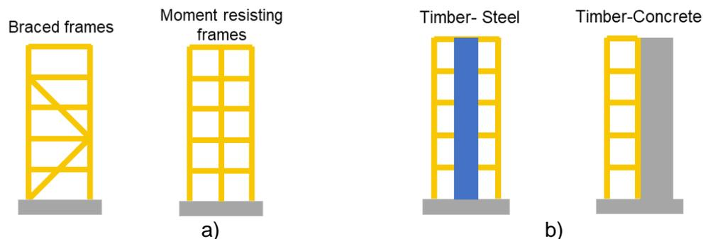
Figure 2: Timber frame LLRSs: brace (left) and moment-resisting (right) frame, (a); Hybrid LLRSs: timber-steel (left) and timber-concrete (right) systems, (b).
