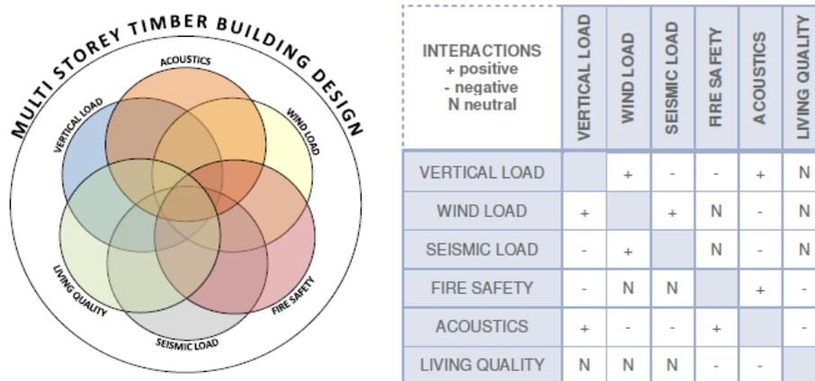
Figure 1: Interaction of a few different building design fields and their inherent collisions, either positive or negative, that need to be resolved for multi-storey taller timber buildings [from Cost Action CA20139 MoU].
