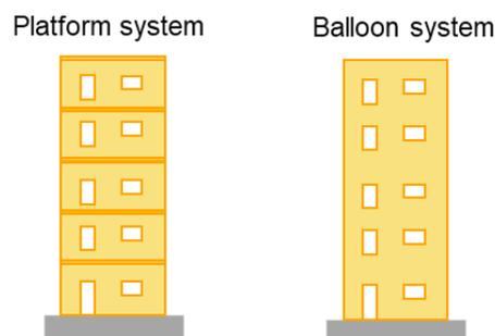
Figure 1: Shearwall construction types: Platform (left) and Balloon (right) system.
