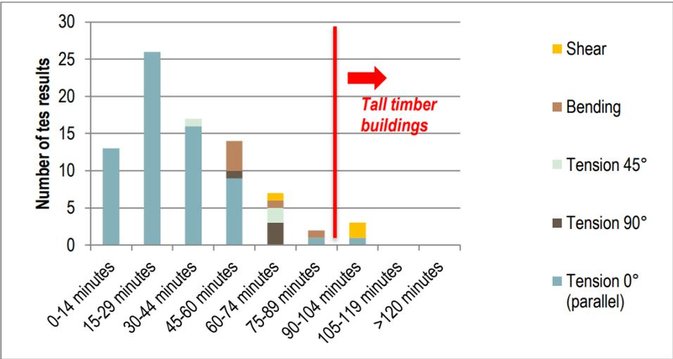
Figure 1: Overview of published fire resistance tests of glulam and sawn timber connections by load direction and fire resistance, from Brandon *et al.* (2019).
