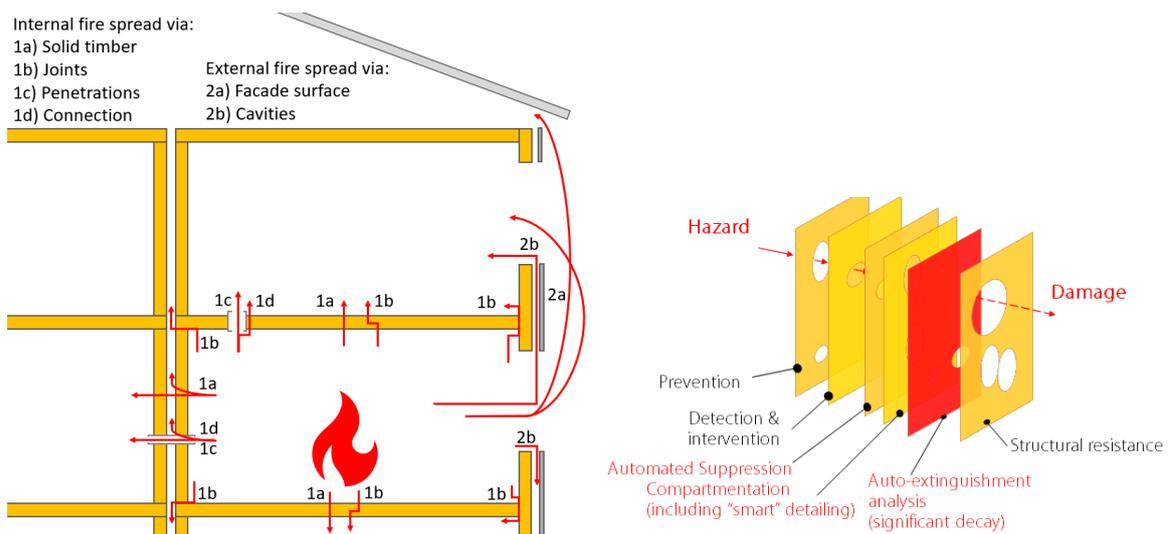
Figure 2: Left, potential paths of fire and smoke spread to be considered (information combined from Brandon *et al.* 2018); Right, visualization of fire safety elements to prevent from damage, modified from Schmid (2022).
