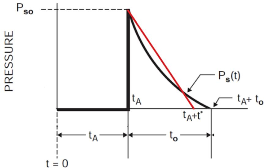
Figure 1: Triangular-shaped curve to model a blast load (adapted from Dusenberry, 2010)
