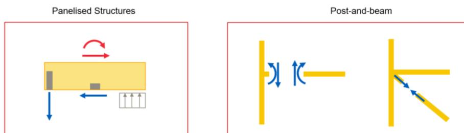
Figure 4: Internal forces in connections of different LLRS for TTB.
